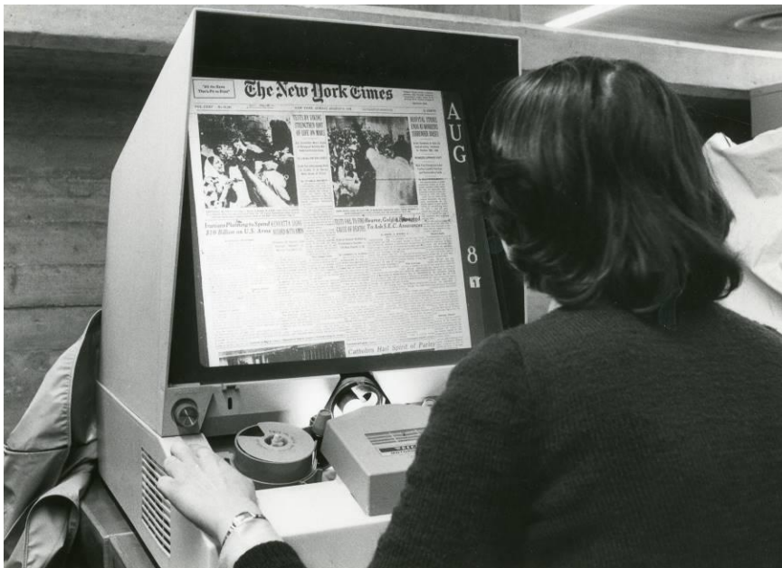
Microfilm readers have been used for decades to view magnified microfilm images.
