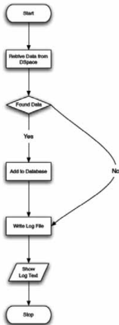
Fig. 17. Flowchart of MobileApp web service document updating process with DSpace.
